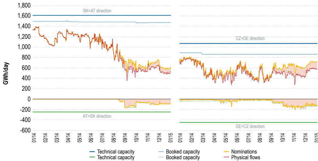
Figure 124: Gas flow developments in Waidhaus (CZ<>DE) and Baumgarten (SK<>AT) in 2014 (GWh/day)
